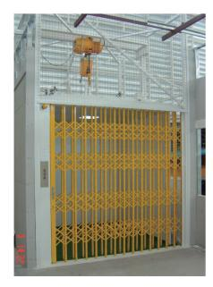
It is simple lift for luggage that corresponds in factory and warehouses, every location. The lifting of Products and parts, the cardboard box, can lift with putting the luggage in the truck or pallet.
